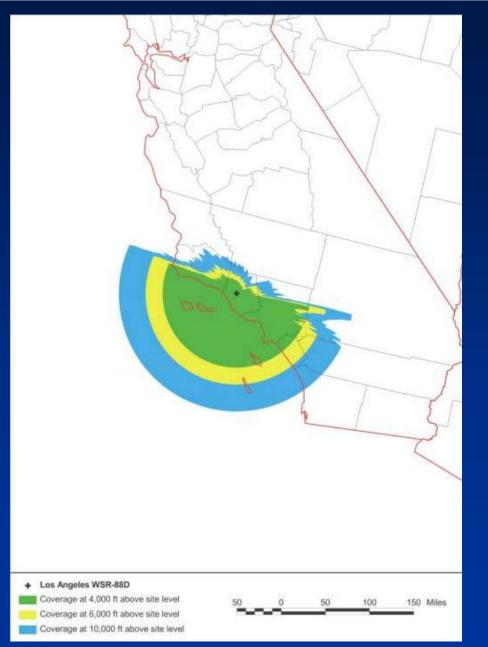
SPAS Example – Complex Terrain and Beam Blockage
