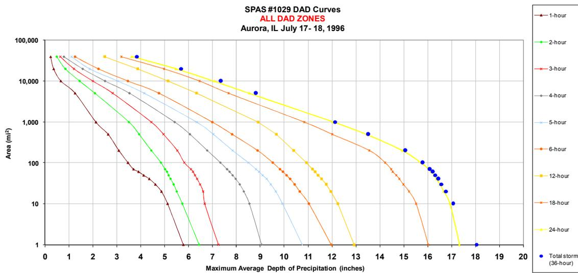
**Figure 1:** Typical DAD plot (a) and corresponding table (b).
