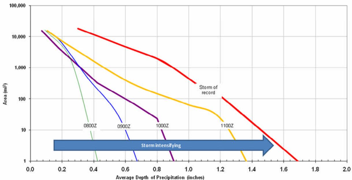
Figure 3. Illustration of four sequential hours of depth-area curves for the 1-hour duration.
